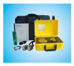
**Growco GDMDFP Series** Doppler ultrasonic flow meter is designed to measure volumetric flow of liquid within closed conduit, the pipe line must be filled full of liquids, there must be a certain amount of air bubbles or suspended solids in liquid.
